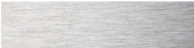
NS Acciaio inox spazzolato AISI 304/Brushed stainless steel AISI 304 Acier inoxydable brossé AISI 304/Acero inoxidable cepillado AISI 304
